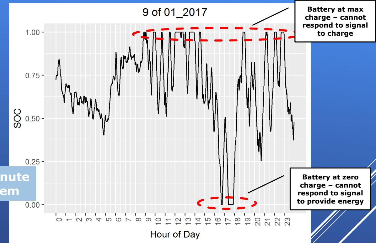
The inability to respond to a signal command to accept more energy from the grid, or give it to the grid, reduced the performance score for what was an optimized storage device prior to the change
