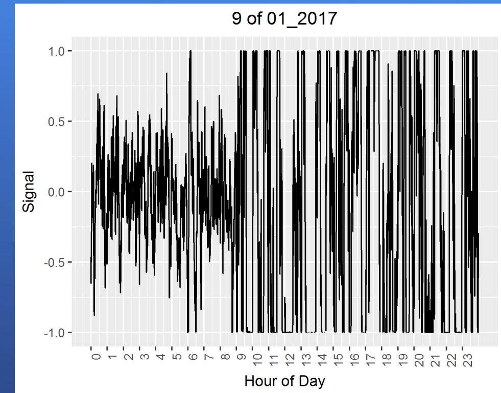
The result of the change to the signal was an increased amount of “pegging” the batteries at full charge or full discharge for “extended” periods of time
